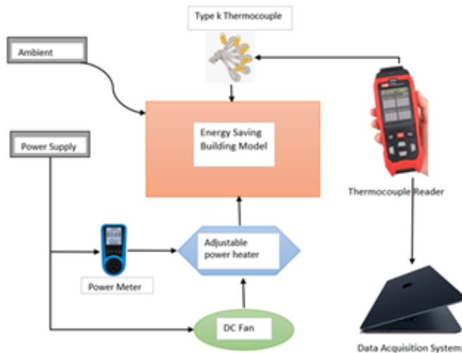
Fig. 2 Schematic diagram of the energy saving building model house
