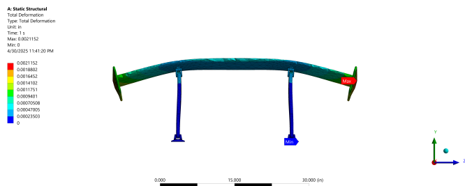
Fig. 4 Total deformation plot of the spoiler under Load Case LC-1 with Aluminum Alloy, shown with a 2 deformation scale factor. Deformation is exaggerated to illustrate bending and displacement characteristics.
