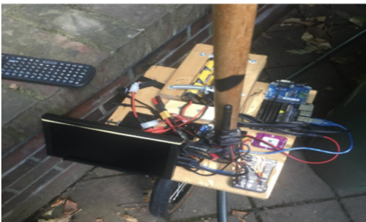
Fig. 7 Portable test stand with PixHawk, GPS, Jetson Nano, and CAN/serial connection to Arduino Due
