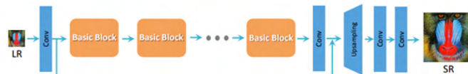
Fig. 1 This figure shows the architecture of the residual in residual dense block (RRDB) 1
