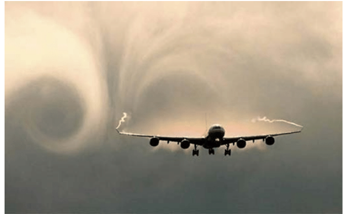
Fig. 1 Rotating vortices in the wake of an airplane 7 .
