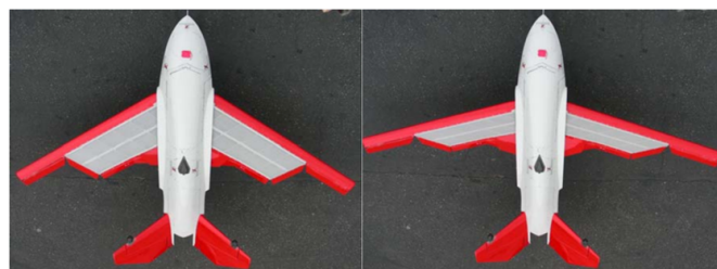
Fig. 7 The wing morphing exhibited by the MX-1. The wings stretched outwards, increasing span and decreasing the wing chord. A flexible wing skin is used to help achieve its morphing 41 .
