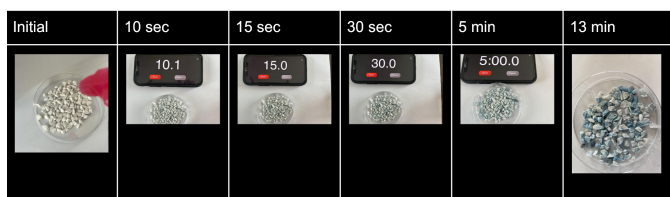
Fig. 4 Time-dependent changes after spraying Leucomethylene blue solution on white drierite.
