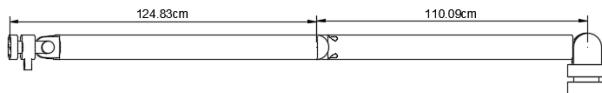
Fig. 7 A horizontal view of the arm stretched out, including basic dimensions in centimeters. Own source created in Fusion 360.
