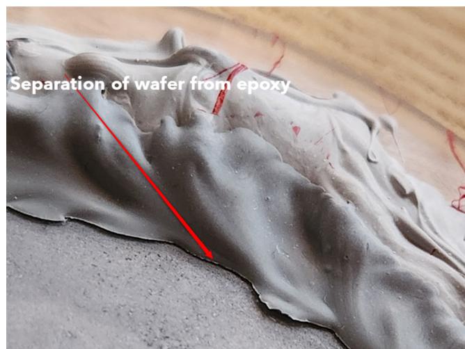
Fig.~ 9 Failure of Photocathode in KOH Electrolyte
