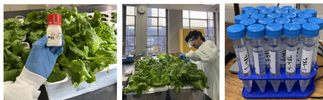
Fig. 4 a) Spiking containers with PFAS chemicals b) Collecting water samples with personal protective equipment (PPE) worn at all times c) Storage of 15 mL water samples to be subjected to PFAS concentration measurement.
