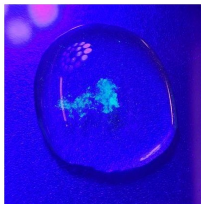
Fig. 3A MP mixed with Mucus using vortex in Part 1 of experiment under UV light
