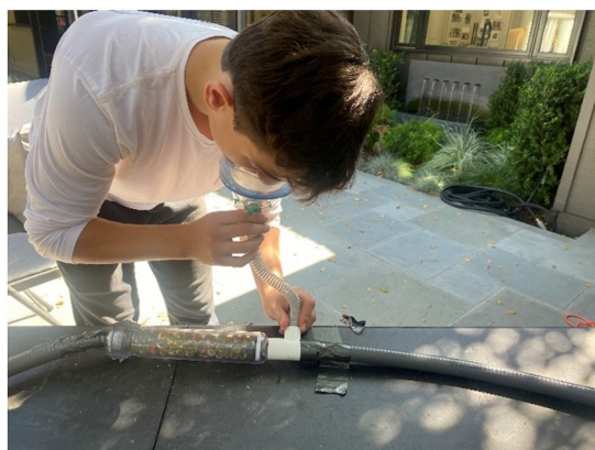
Fig. 5 Olfaction test: 2 second evaluation of smoke for Syringol. Likert 1= odorless; 5 = strong sweet (or pleasant) smell
