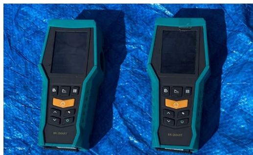
Fig. 4 2 TVOC/PM 2.5 meters (BLATN BR-smart 128s) located at the terminal end of the hoses.
