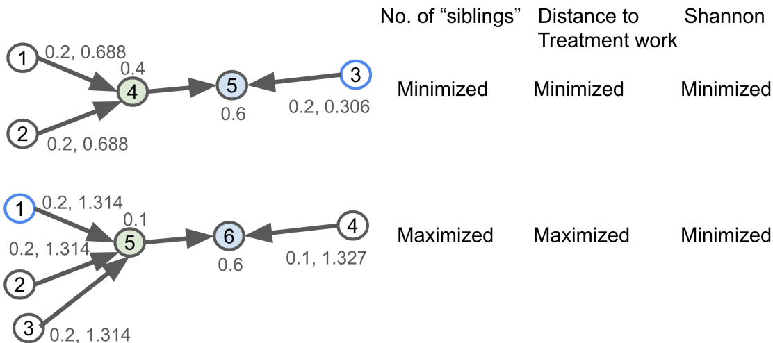
Fig. 4 Lack of consistency of alternative parameters number of siblings (buildings that share the same immediate sewage intersection) and distance between a building and a treatment work for Shannon entropy with optimal building in blue
