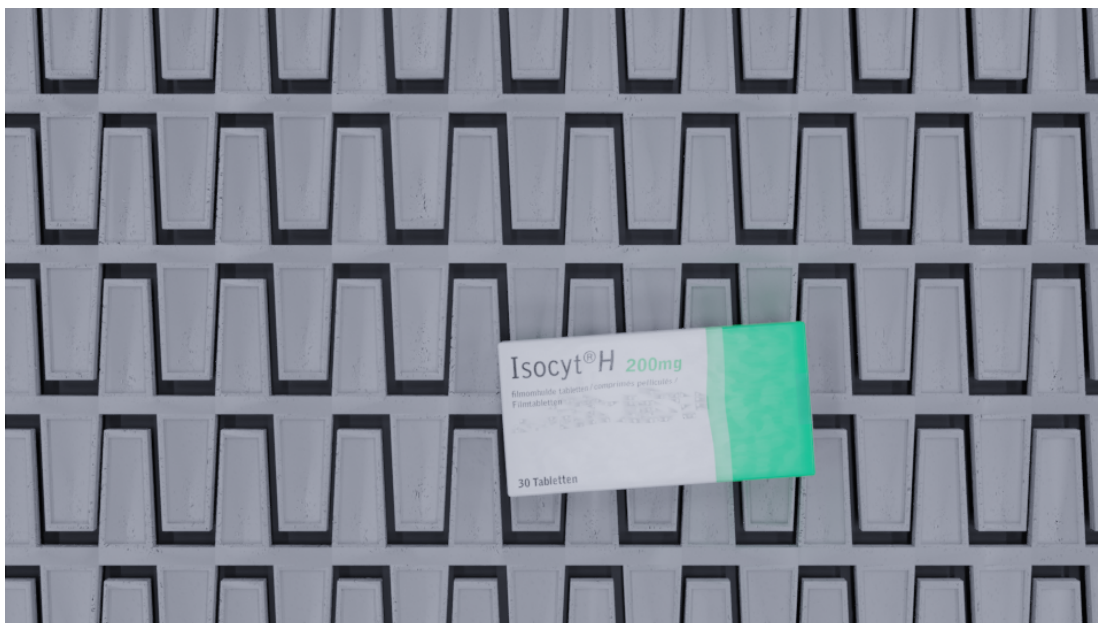
Fig. 4 A package image from the top view that is damaged despite looking intact.
