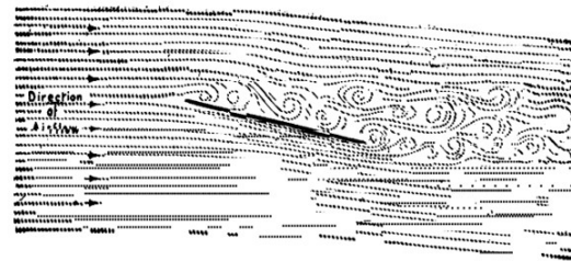
Fig. 25 The above diagram shows the airflow over a flat plane. The presence of the vortices along the upper surface of the plane reveals that flow separation has led to a loss in lift efficiency. An ideal model would display two synchronized airflows and the elimination of the vortices. A similar characteristic can be observed in airfoils whose angle of attack exceeds its most efficient state 2 . (Image taken from Flight Without Formulae)
