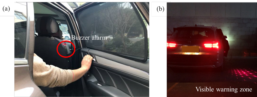
Fig. 8 Prototype Test Show. (a) Buzzer alarm to alert passengers not to open the door. (b) The laser light emits a red beam which creates a distinct warning area on the ground.
