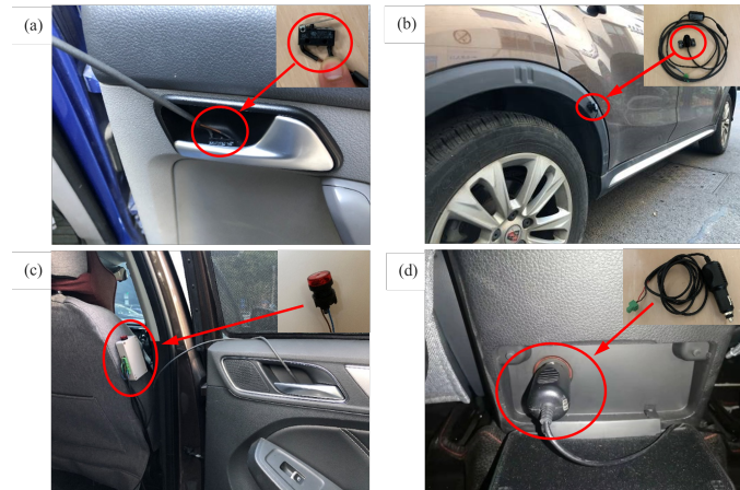
Fig. 4 Hardware installation (a) Microswitch inside the door handle. (b) Laser light on the right rear fender. (c) Buzzer beside B pillar inside. (d) Socket plug connector.
