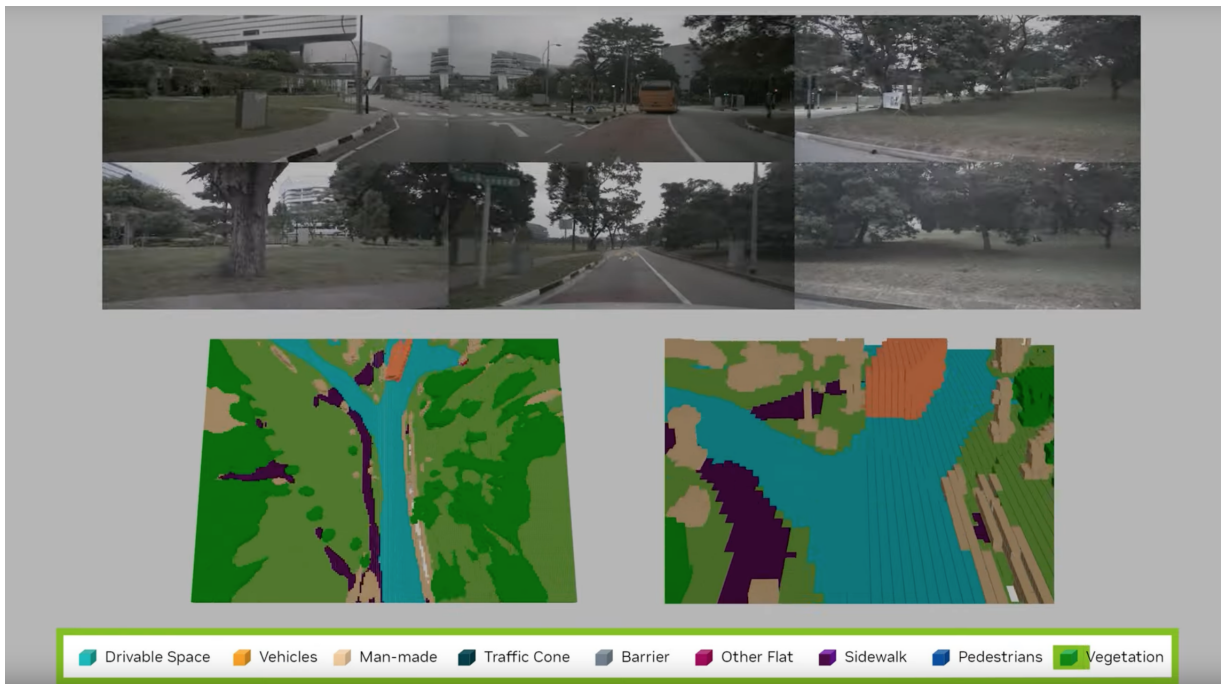
Fig. 5 NVIDIA wins the 3D Occupancy Prediction Challenge with FB-OCC, a technology designed for using camera data to generate 3D voxel bird's-eye maps. The bottom two maps exemplify the creation of voxel grids using sensor data from the six camera inputs above 23 .
