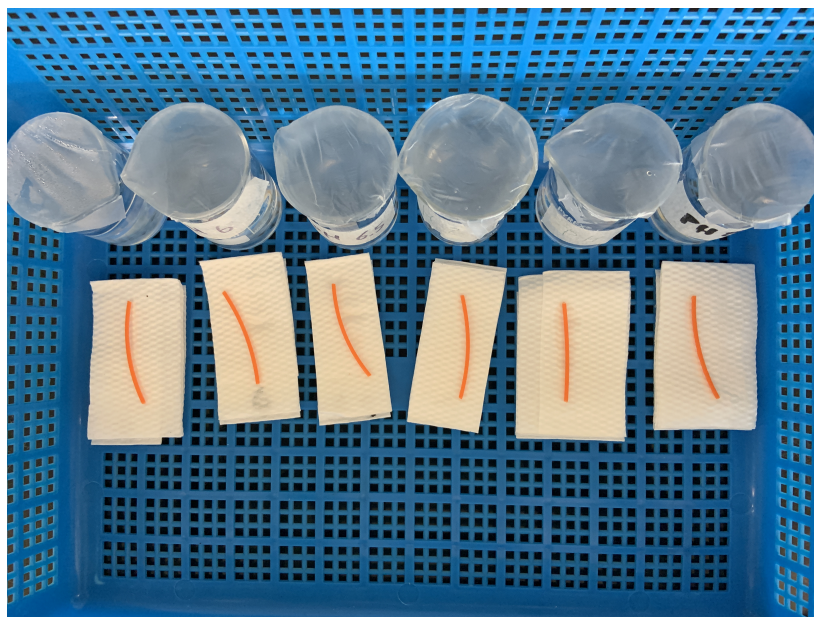
Fig. 3 Strips of PLA drying inside of the fume hood next to their respective phosphate buffers
